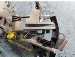
9. Using Dremel or similar tool grind shifter assembly as shown to allow shifter detent to move further up into shifter assembly. (The long side of the curved opening will typically need to be extended to the point where the assembly starts to bend)
