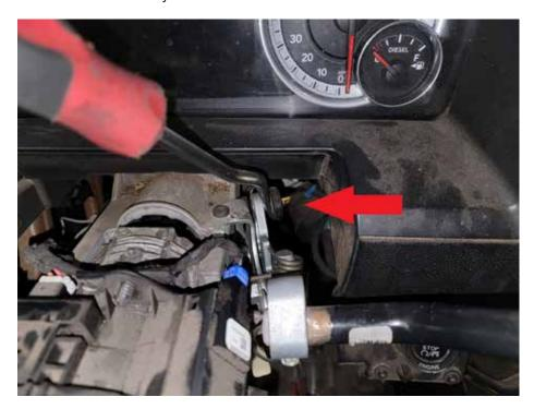
**7.** Remove (3) T27 bolts holding shifter assembly to steering column and remove from vehicle.
